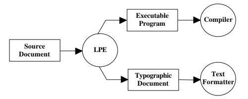
A source document of the literate program is created in the LPE. The LPE uses two different processes to generate an executable program document and a typographic document from the source document. These documents is respectively executed by a compiler, and printed with a text formatting tool.
