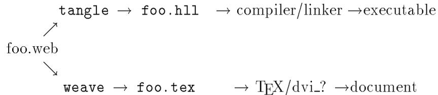
**Figure 1.** The WEB process. The source of the code and documentation are in the source file `foo.web`. The `tangle`, compile, and link process creates an executable. The `weave`, T<sub>E</sub>X, and dvi conversion process creates a document.
